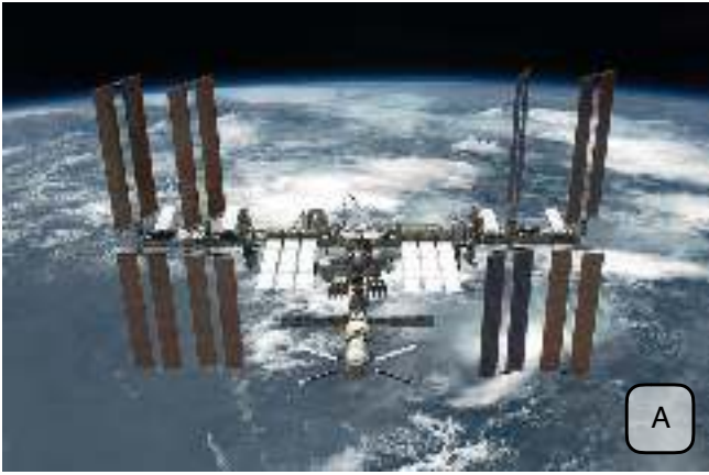
FIGURE 3 : (A) Photograph of the International Space Station (ISS) in Earth orbit. It has dimensions of 110x74x30 (LxWxH in meters) and a total mass of 400 tonnes, its autonomous operation is provided by eight solar generators. Each consists of a mast surrounded by two 32m x 11m surfaces that support the photovoltaic cells. (B) Dome simulating life on Mars during the HI-SEAS program that took place on the slopes of the Kilauea volcano in Hawaii. The living conditions and thus the energy requirements for the autonomy (essentially pressurization and heating) of this Mars colonization module are similar to those of ISS.
